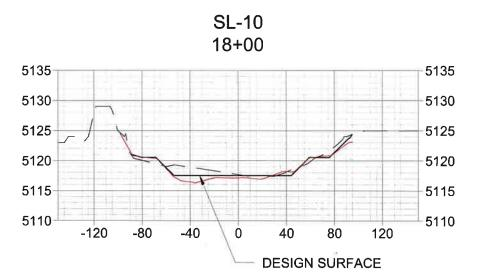
NOTE: AS-BUILT SURVEY SHOWN ON CROSS SECTIONS BASED ON FIELD SURVEY COMPLETED BY CEPI 5/20/2016. DEEP POOLS WILL BE SURVEYED IN THE FALL OF 2016. UPDATED AS-BUILT WILL BE DELIVERED WHEN AVAILABLE.
